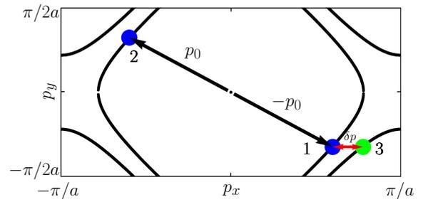
**Figure 14.** Brillouin zone and Fermi surface (black curves) of the AF layer. Zero-momentum Cooper pair between electrons 1 and 2 is schematically shown by black arrows. There is also Néel-type finite-momentum triplet pairing between electrons 2 and 3, which is produced from electron 1 due to the Umklapp reflection process from the S/AF interface. The total momentum  $\delta p$  of the pair (2 and 3) is shown by the red arrow. The picture is adopted from Ref. [76].
