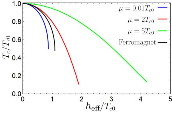
**Figure 5.** Critical temperature of the S/AF bilayer as a function of  $h_{\text{eff}}$  for different values of  $\mu$ . Black line represents the dependence  $T_c(h_{\text{eff}})$  for an S/F interface with a ferromagnetic insulator producing the same value of the effective exchange field (but homogeneous, not staggered) in the superconductor. The picture is partially overlapped with an analogous picture from Ref. [34].
