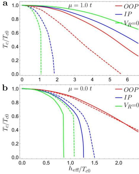
**Figure 30.** **a, b** – Critical temperature of S/AF (solid curves) and S/F bilayers (dashed) as a function of the effective exchange field  $h_{\text{eff}}$ . Panels **a** and **b** correspond to  $\mu = 12T_{c0}$  and  $\mu = 0$ , respectively. Green curves represent the results with no SOC, red and blue curves are for out-of-plane (OOP) and in-plane (IP) orientations, respectively, and  $V_R = 0.4t$  is the Rashba SOC strength. The picture is adopted from Ref. [119].
