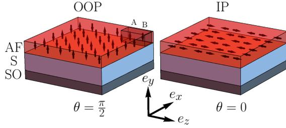
**Figure 29.** Sketch of the thin-film S/AF bilayer with SOC. The Néel vector of the AF makes angle  $\theta$  with the plane of the structure.  $\theta = 0$  corresponds to the in-plane (IP) and  $\theta = \pi/2$  accounts for the out-of-plane (OOP) orientations. Unit cell with two sites A and B is also shown. The picture is adopted from Ref. <sup>119</sup>
