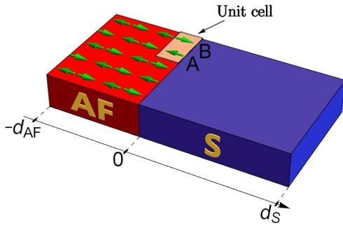
**Figure 16.** S/AF bilayer with a finite-width metallic AF. Staggered magnetization of the AF layer is schematically depicted by arrows. The unit cell containing two sites belonging to A and B sublattices is also shown. The picture is adopted from Ref. [76].
