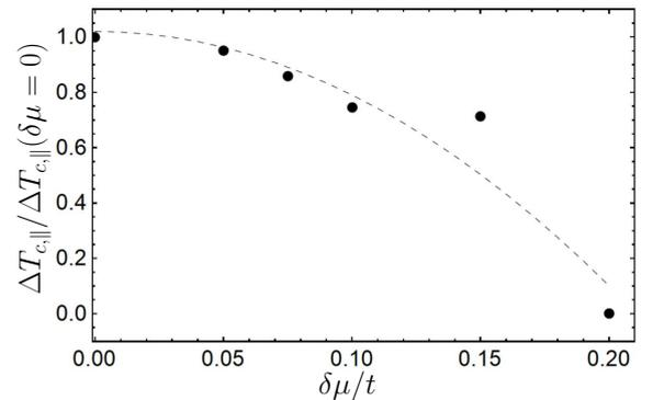
**Figure 24.** Suppression of the spin-valve effect by impurities. The difference  $\Delta T_{c,\parallel}$  is plotted as a function of the impurity strength  $\delta\mu$ . The difference is normalized to its value at  $\delta\mu = 0$ . The dashed line is a guide for the eye. All calculations were performed for the following parameters:  $\mu_S = 0.9t$ ,  $\mu_{AF} = 0$ ,  $h = t$ ,  $d_{AF} = 4$  and  $d_S = 20$  monolayers, and  $T_{c0} = 0.03t$ . The picture is adopted from Ref. [78].
