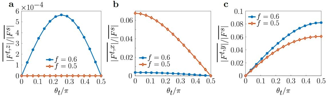
**Figure 7.** **a, b, c** – Variations of the triplet correlations with the canting angle  $\theta_t$  for different filling factors  $f = 0.5$  ( $\mu = 0$ ) and  $f = 0.6$  ( $\mu/T_{c0} \approx 65$ ). These panels show the average magnitudes of the normalized spin-triplet correlation  $F^{t,z}$  (panel a),  $F^{t,x}$  (panel b), and  $F^{t,y}$  (panel c). The averages are taken over all superconducting sites and they are denoted via an overhead bar. The picture is adopted from Ref. [39].
