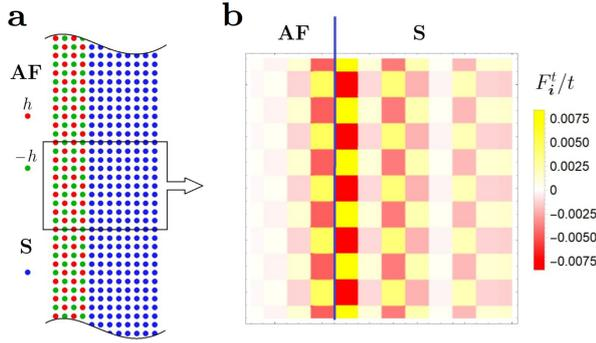
**Figure 1.** **a** – Sketch of the antiferromagnetic insulator with a compensated interface attached to the thin superconductor. **b** – Spatial variation of the amplitude  $F_i^t$  of the triplet correlations. Each colored square codes the value of  $F_i^t$  at a given site. An alternating sign of the correlations in S-layer commensurates with the Néel order in the AF-layer along the interface direction. The picture is adopted from Ref. [34].
