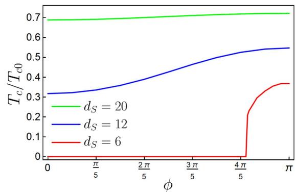
**Figure 21.** Dependence of  $T_c$  on the misorientation angle  $\phi$  for the AF/S/AF structure at half-filling ( $\mu_S = 0$ ). Different curves correspond to the different  $d_S$  values (all widths are measured in the number of monolayers). All calculations were performed for the following parameters:  $d_{AF} = 4$ ,  $\mu_{AF} = 0$ ,  $h = 0.5t$ , and  $T_{c0} = 0.07t$ . The picture is adopted from Ref. [78].
