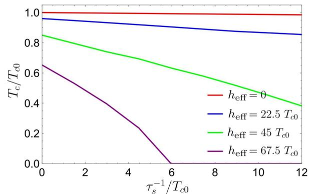
**Figure 12.** Dependence of  $T_c$  on  $\tau_s^{-1}$  at  $\mu = 150 T_{c0}$  for different effective exchange fields  $h_{\text{eff}}$ . The picture is adopted from Ref. [38].
