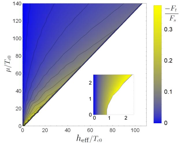
**Figure 4.** Amplitude of the triplet correlations relative to the singlet amplitude as function of  $h_{\text{eff}}$  and  $\mu$  at  $T \rightarrow T_c$ . Inset: region  $(h_{\text{eff}}, \mu) \sim T_{c0}$  on a larger scale. The picture is adopted from Ref. [38].
