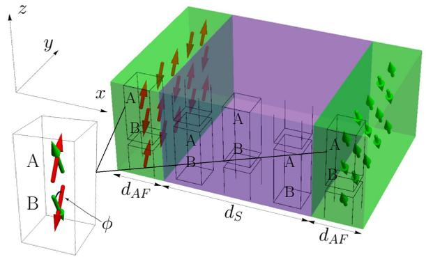
**Figure 20.** Sketch of the AF/S/AF system. Red and green arrows show Néel-type magnetizations of the AF-layers. The unified division into two sublattices with unit cells containing two sites belonging to A and B sublattices is also shown. The misorientation angle  $\phi$  is defined as the angle between the magnetizations of two antiferromagnets at the same sublattice. The picture is adopted from Ref. [78].
