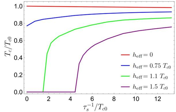
**Figure 11.** Dependence of  $T_c$  on  $\tau_s^{-1}$  at  $\mu = 0$  for different effective exchange fields  $h_{\text{eff}}$ .  $T_c$  is normalized to the value of the critical temperature  $T_{c0}$  of the isolated S-film. The picture is adopted from Ref. [38].
