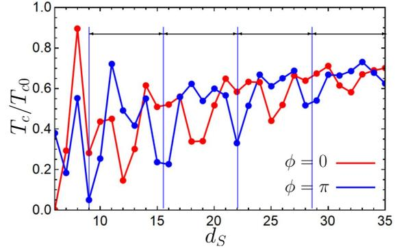
**Figure 23.** Dependences  $T_c(0)$  and  $T_c(\pi)$  as functions of  $d_S$  at  $\mu_S = 0.9t$ . The calculations were performed for the following parameters:  $d_{AF} = 4$ ,  $\mu_{AF} = 0$ ,  $h = t$ , and  $T_{c0} = 0.03t$ . The period of the oscillations is  $L_{\text{osc}} = \pi v_F/\mu_S \approx 7$ . Four periods (minima  $T_c(d_S)$  for  $\phi = \pi$ ) are shown on the plot by vertical blue lines. The picture is adopted from Ref. [78].
